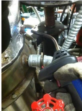
*Figure 6: Light the Gasifier, Step 3*
