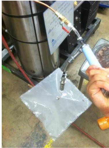
*Figure 10: Collect the Syn-Gas, Step 7*
