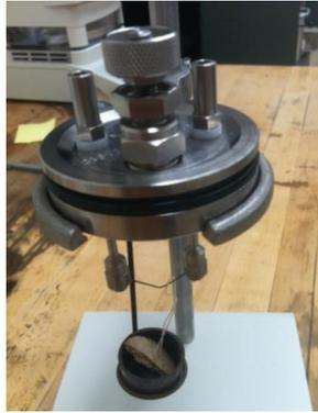
*Figure 1: Attach Cotton Thread*
