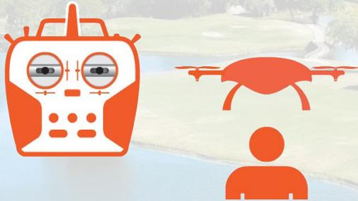
Rotation around the front-to-back axis is called **roll**. – Right stick left or right
