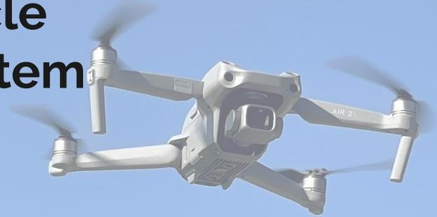
An unmanned aircraft system is an unmanned aircraft and the equipment necessary for the safe and efficient operation of that aircraft. An unmanned aircraft is a component of a UAS. It is defined by statute as an aircraft that is operated without the possibility of direct human intervention from within or on the aircraft.
