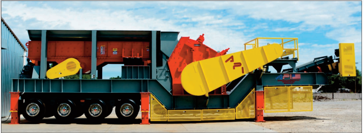
FIGURE 5: Primary Crusher Station. Hazemag Horizontal Impact Crusher on a Chassis. (Courtesy, Aggregate Processing, Inc.)
