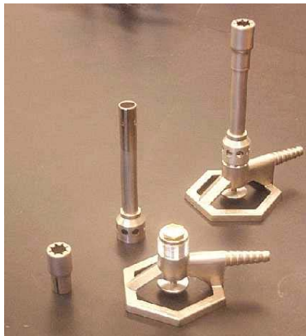
Burner stack and base (foreground), and fully assembled burner.
